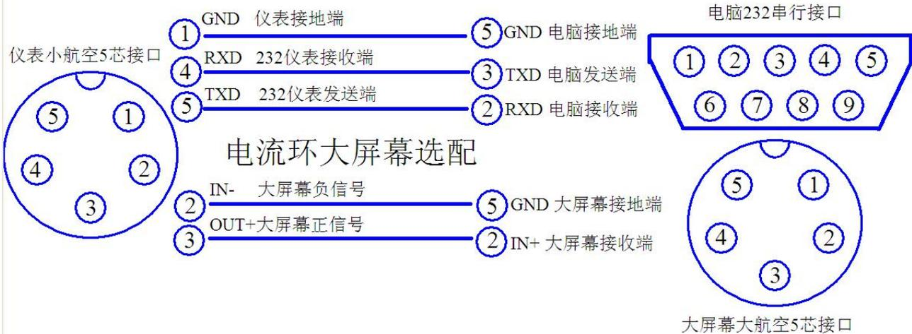
(Figure 2-4) Diagram of connection between instrument and computer and large screen
